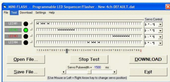
Probably the neatest feature of the Mini-Flash is the ability for the user to completely customize the flashing sequence for each of the 4 LED channels, and then download it to the Mini-Flash. Not only are these sequences programmable, but the user can also program the overall LED sequencing speed. Another really neat and very
