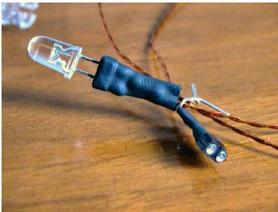
DIYRC also sells machine pin connectors for simple plug-in of LEDs. Only apply heat shrink around the metal portion of the connectors and connecting wires, especially on the connector side that will connect to the Mini-Flash controller. (see picture on left). These two-pin machine pin connectors allows for the user to replace LEDs (maybe to simply change a color). The LED connector include a 100 ohm resistor (inside the black heat shrink tubing). Just a
