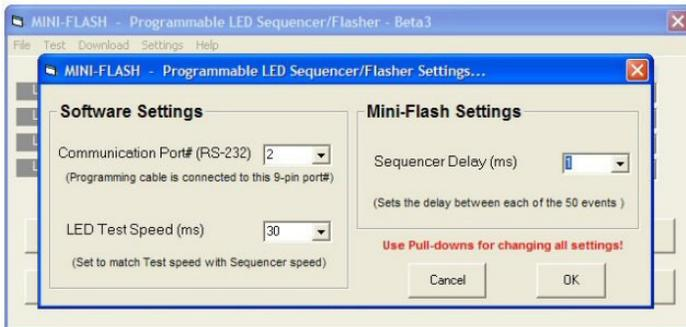
The Mini-Flash programming software allows the user to alter the Mini-Flash sequencer speed. Additionally, the software also allows the user to select the proper communications port to which the download cable is connected. These settings can be changed by selecting the "Settings" menu option.
