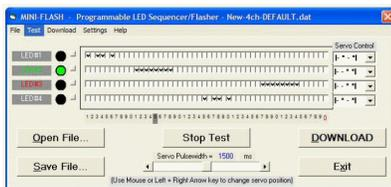
**Step 4:** Now, run the software and configure the LED channels as you like them. You could also load a supplied example file for test purposes. If you haven't done so already, you could "virtually" test the sequence by hitting the "Test" button in the software (hit "Stop Test" button to
