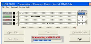
**Step 7:** You will notice that immediately after you hit the "OK" button, Mini-Flash's LEDs all go out (all LED extinguish). At the same time, you will see the downloading progress as indicated by the software's download progress bar along the bottom of the screen.
