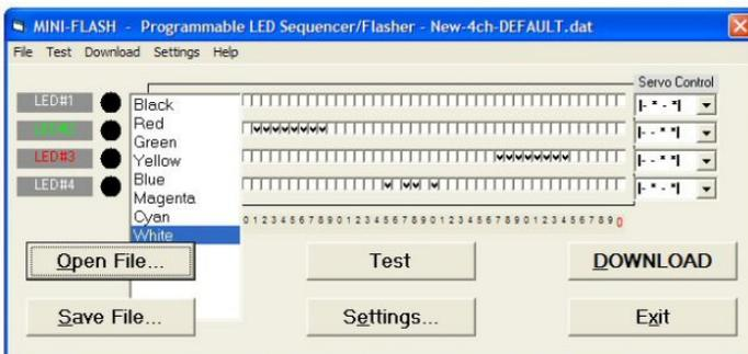
The Mini-Flash programming software emulates the LEDs connected to the Mini-flash controller and these LEDs (LED#1 - 4) are shown towards the left of each of the 4 sequence event rows. Initially, when the software is loaded, these color
