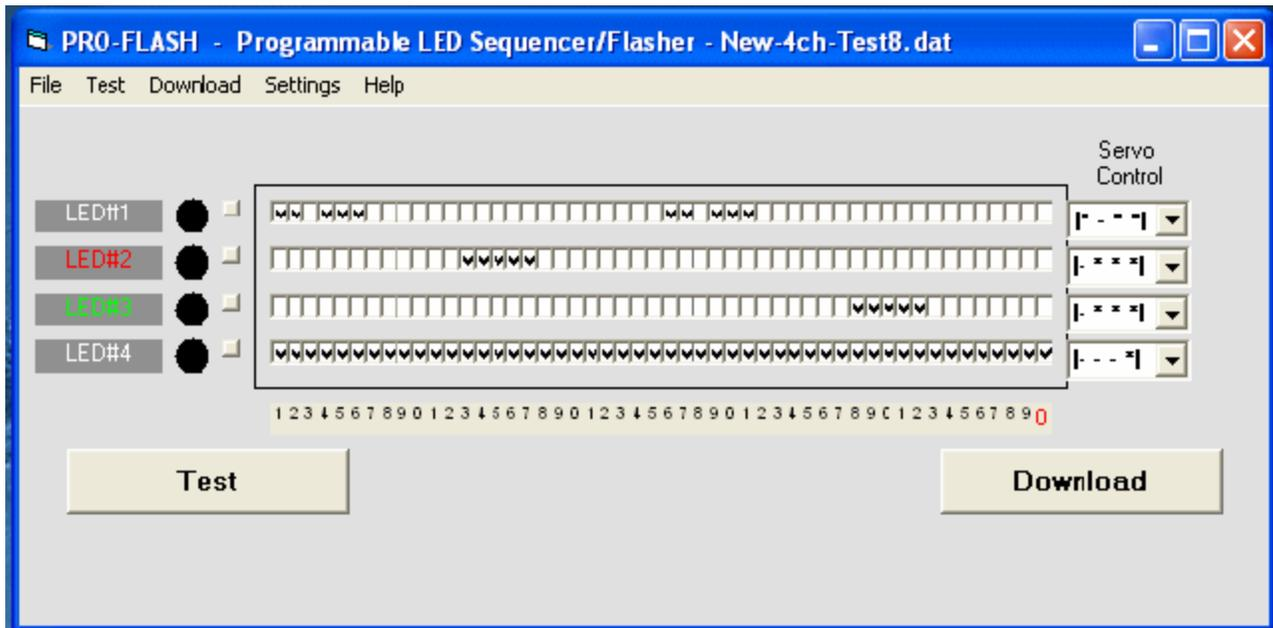
As for servo controls, the following can also be programmed (assuming you are controlling Mini-Flash using a spare slider/stick channel, or even tapping off of the throttle servo wire):
