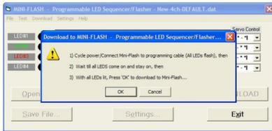
**Step 5:** When happy with the sequence and controls, hit the "Download" button and a message (shown on left) will pop up. This message tells you to cycle power to the Mini-Flash or connect the Mini-Flash to the programming cable. **STOP! The next step (#6) is very important so please**
