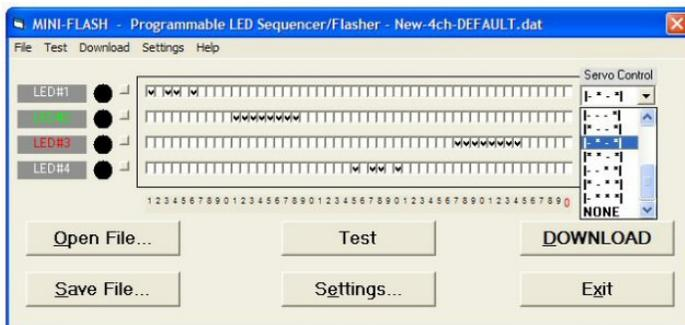
The Mini-Flash programming software includes a "servo control" for each of the 4 channels that allows the user to use a R/C servo output (from a R/C receiver) as a "switch" control for each LED channel. This feature allows the user to control (turn On or Off) each of the 4 channels in
