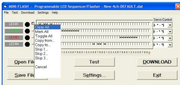
The Channel Options button allows you to manipulate the selected channel's sequence in that you can quickly:
