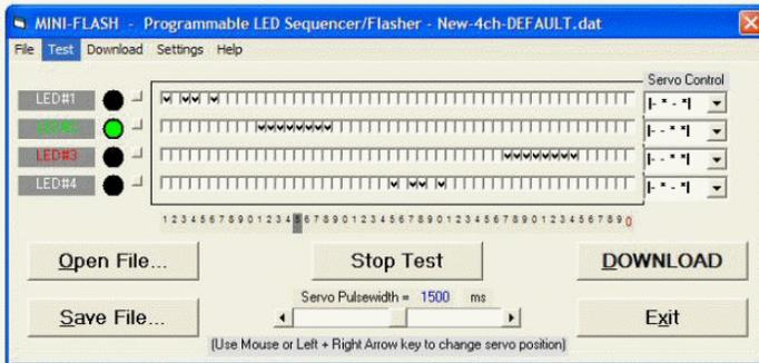
The programming software allows the user to "test" the current programmed sequence, including the servo control functions programmed by the user. To initiate the test, press the "Test" button in the programming software. Upon pressing this button, you will see the test sequencer display the programmed sequence on the graphical LEDs in the
