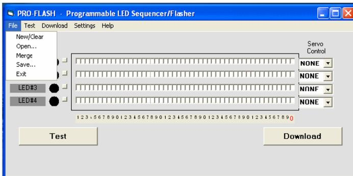
The programming software allows the user to either develop a **New** LED sequence (clearing all current sequence events), **Open** an existing sequence file (previously saved sequence files like the sample files included), **Merge** an existing sequence file into the currently displayed sequence or **Save** the current sequence. These options are easily
