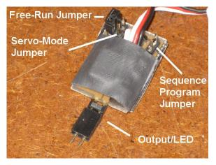
The Mini-Beacon controller has a servo cable which can either be plugged into a spare channel on your Radio Control receiver (Rx) or it can simply be connected to a 5-6 volt power source. Opposite of this servo cable lies a two pin connector (inline with board) that is used to connect your beacon LED. The onboard output driver/transistor is capable of providing around 600mA to a connected load (same output voltage as input). A typical 5mm LED draws 20mA while a 1 watt Luxeon emitter draws an
