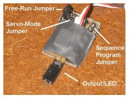
2) While the pattern is flashing, continuously short the programming jumper (two pins shown towards the top/right on drawing) with either the supplied jumper or a piece of conductive metal (coin, paper clip, screw/nail, etc...)
